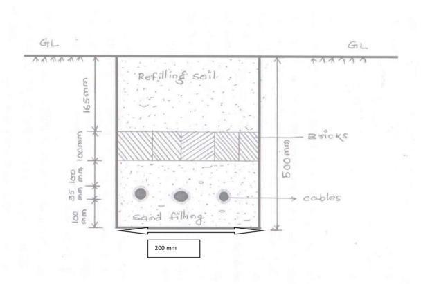
Note:-Wherever bricks are not available the cables must be buried between two layers of sand
